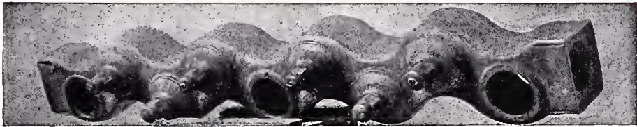
Babcock & Wilcox Manifold Header, forged from Steel.
